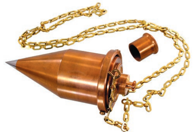
The catalog listed this plumb bob with the seldom-used superlative of "in brand new, unused condition." Made by the Heller & Brightly Company of Philadelphia, it was used for sighting in dark mine shafts. Heller & Brightly was a small craft workshop with only a few employees, each of whom was capable of producing an entire tool. They built only about 100 implements per year between 1870 and 1887, with production peaking in 1891 at 216 units. Stamped on the side "HELLER & BRIGHTLY / PHILAD.," the rare and pristine instrument fell at $1380 (est. $800/1600).
