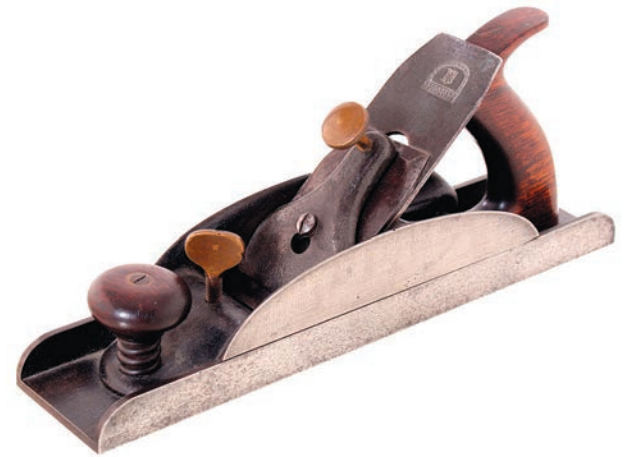
Metallic transitional planes by the prolific Massachusetts inventor Leonard Bailey (1825-1905) were prized by his contemporary woodworkers for their durability and precision craftsmanship. They still are, as well as for their rarity. This one is a variation on the split-frame theme, as illustrated in Roger Smith's Patented & Transitional Metallic Planes in America: 1827-1927 . It missed the $10,000/20,000 target and sold for $7590.
